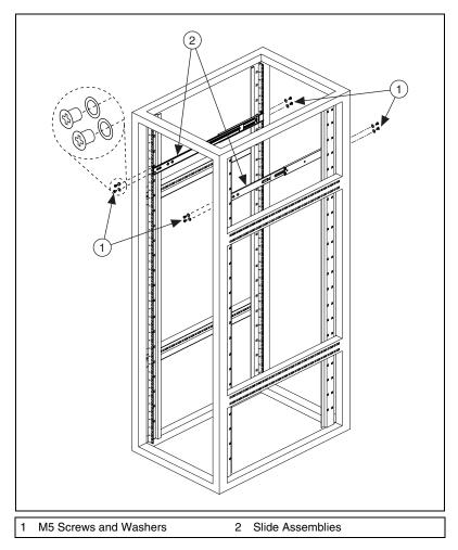
Figure 2-3. Installing Slide Assemblies into Rack
